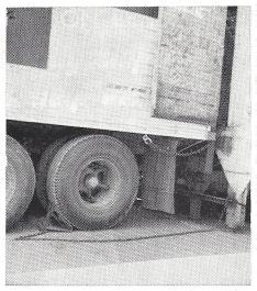
SAFETY CHOCK AND CHAIN IN BUSINESS—Note safety chock behind rear wheel of this truck and steel chain above which fastens firmly to loading dock. This truck can't move to cause possible injury!
